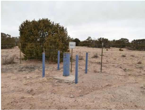
Figure 2-9. Groundwater Monitoring Well
