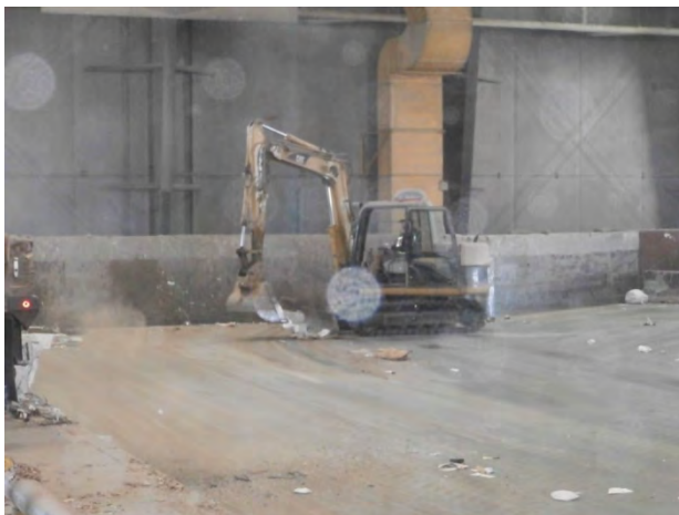
Figure 3-7. Excavator Used to Pack Transfer Trailers
